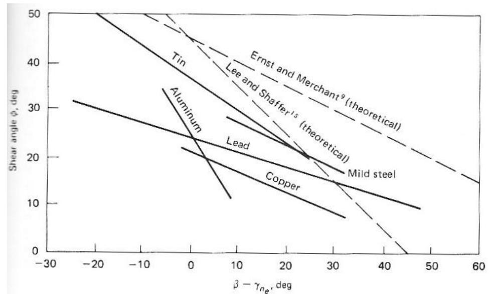
Figure 2.18 Comparison of theoretical and experimental shear-angle relationships for orthogonal metal cutting, where  $\phi$  = shear angle,  $\beta$  = mean friction angle on tool face, and  $\gamma_n$  = working normal rake. [After Pugh [19].]
