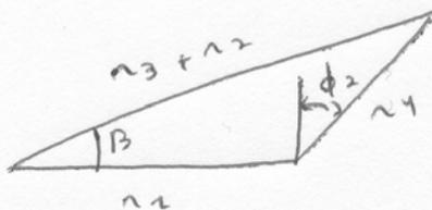
$$(r_3 + r_2) \cos \beta = r_1 + r_4 \sin \phi_2$$
