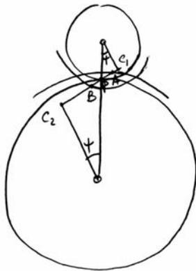
$$\overline{AP} = \overline{AC_2} - \overline{PC_2} = \sqrt{(R_2 + a)^2 - (R_2 \cos \varphi)^2} - R_2 \sin \varphi$$
