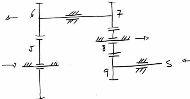
$$\frac{\bar{w}_s}{\bar{w}_t} = -\frac{z_5 z_7 z_8}{z_6 z_8 z_9} = -\frac{50 \times 30}{90 \times 70} = -\frac{15}{63} = \frac{w_s - w_t}{w_s - w_t}$$
