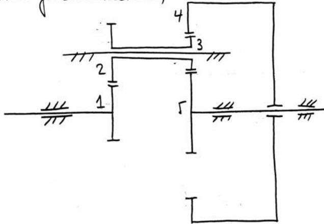
$$\textcircled{1} \frac{\bar{w}_s}{\bar{w}_e} = \frac{z_1 z_3}{z_2 z_5} \Rightarrow \frac{w_s - w_t}{w_e - w_t} = \frac{26 \times 22}{32 \times 36}$$
