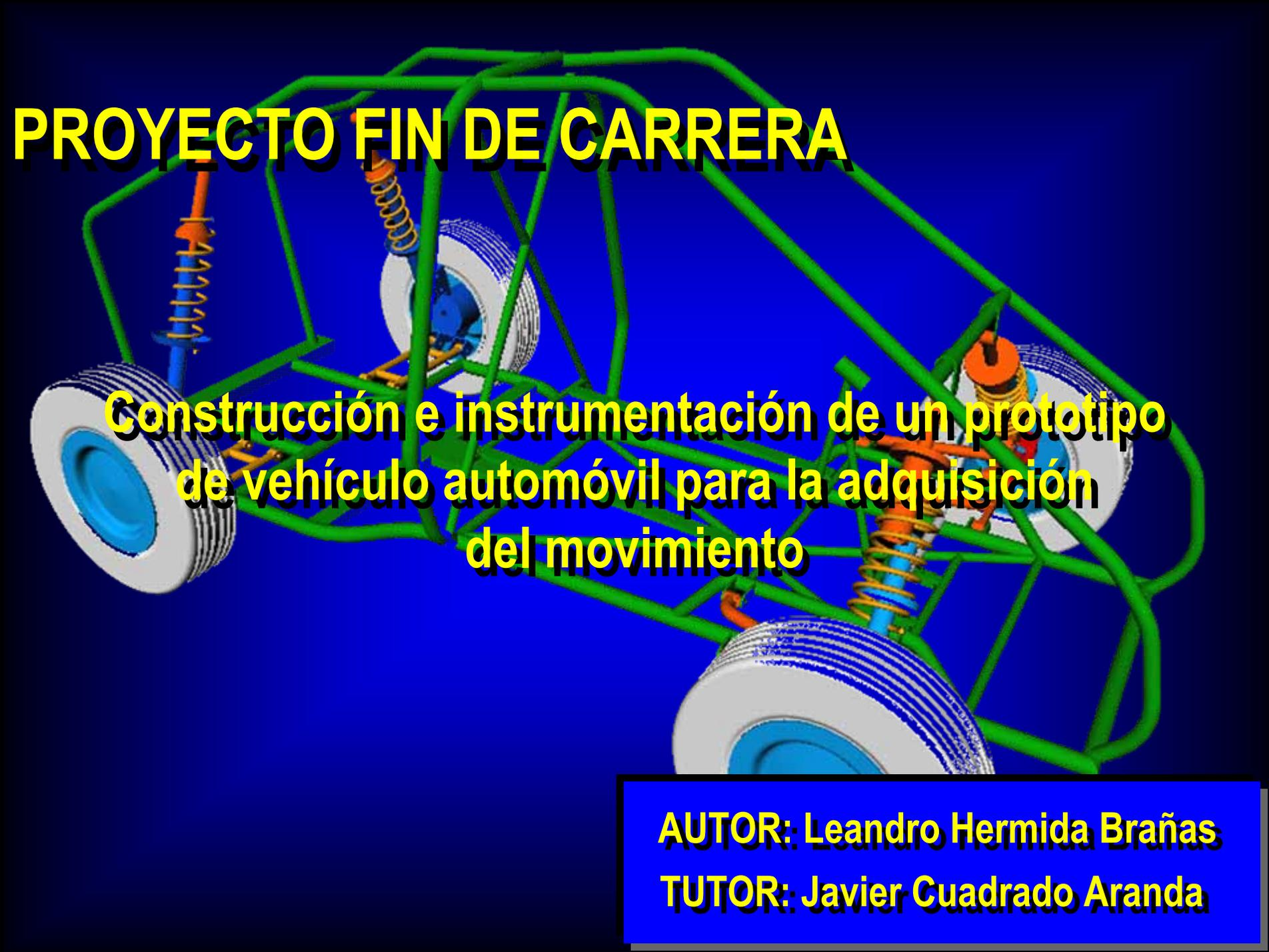
A 3D CAD model of a vehicle chassis, rendered in green. The model shows a complex frame with four wheels, each with a blue tire and a white hub. The suspension system is visible, featuring blue coil springs and orange shock absorbers. The entire model is set against a solid blue background.
