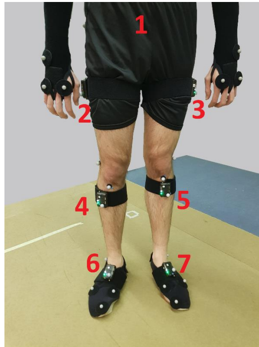
Figure 3. Markers and IMUs (red numbers) attached to the subject's body for gait analysis.
