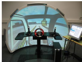
Fig. 4 – Human-In-The-Loop simulators of excavators
