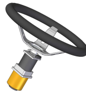
Fig. 13 – CAD model of the steering wheel system
