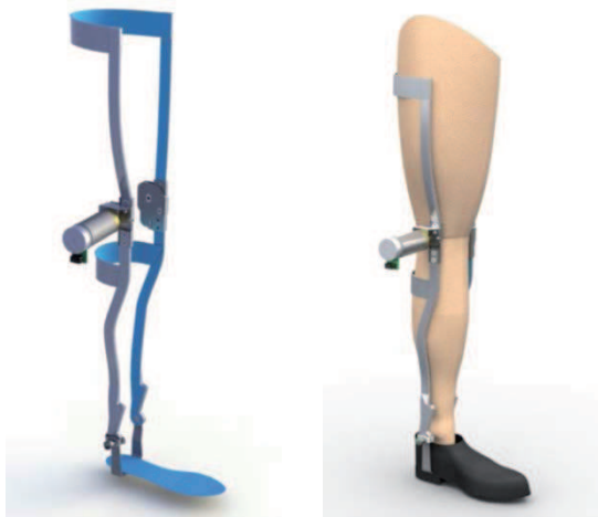
Figure 2. Global mechanical design of the orthosis.
