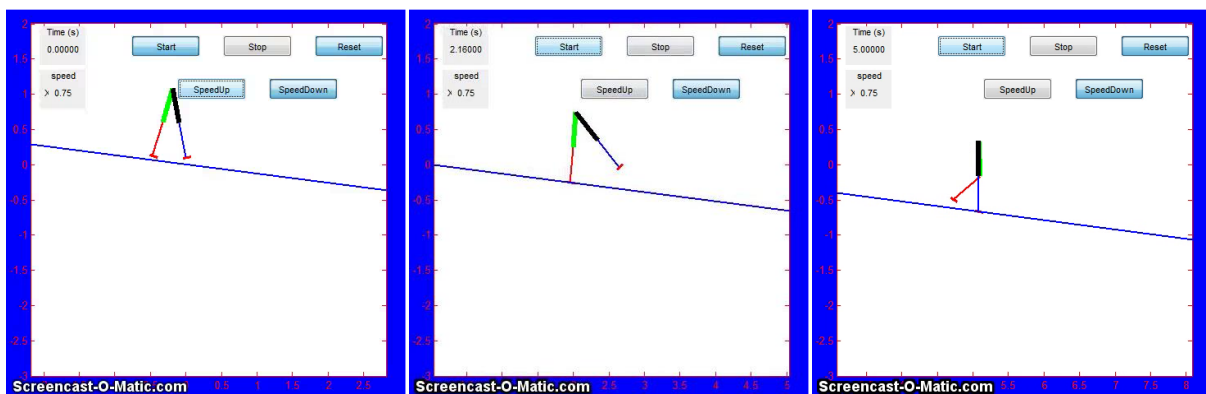
Figure 1. Snapshot of dynamic simulation of bipedal robot walking with multi-point foot contact
