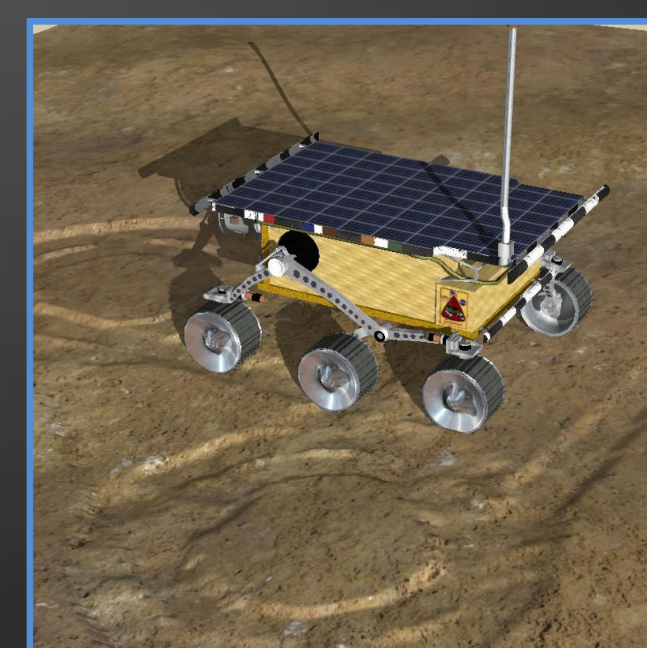
High-fidelity model in Vortex with soil compaction and hardening
